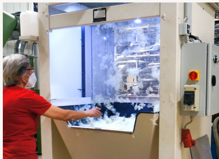
Nonwoven recycling plant – fiber recovery from nonwoven waste
